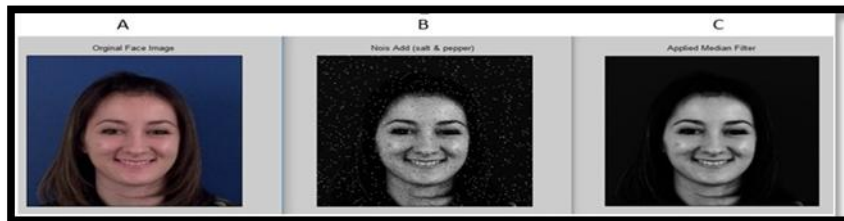
Figure (2): Image Pre-Processing Steps (A), Input image (B) Noise Add, (C) Median Filter Apply.
